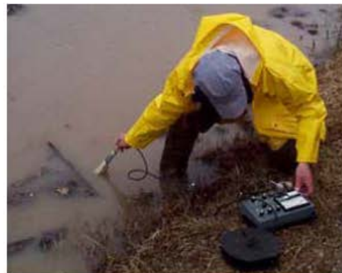
Testing for dissolved oxygen in a flooded farm field with spoiling sugar beets.
