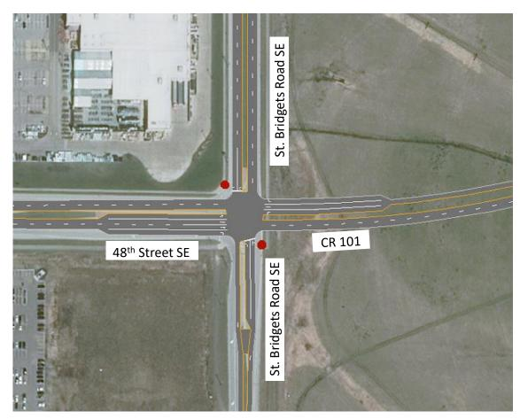
Install Two Way Stop Control for Northbound and Southbound St. Bridgets Road SE
