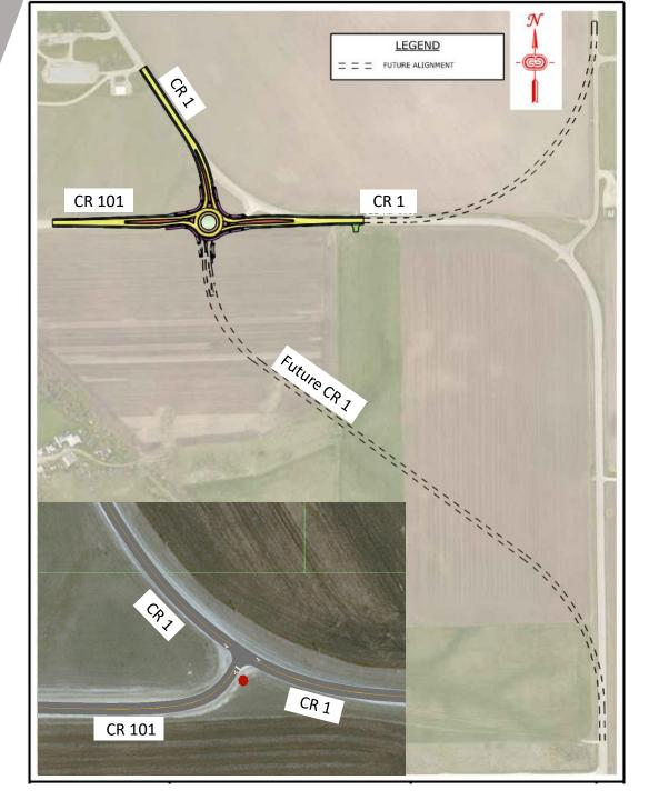
A roundabout is recommended to improve geometrics at the intersection with this project and to set the stage for eliminating substandard horizontal curves in the future.
