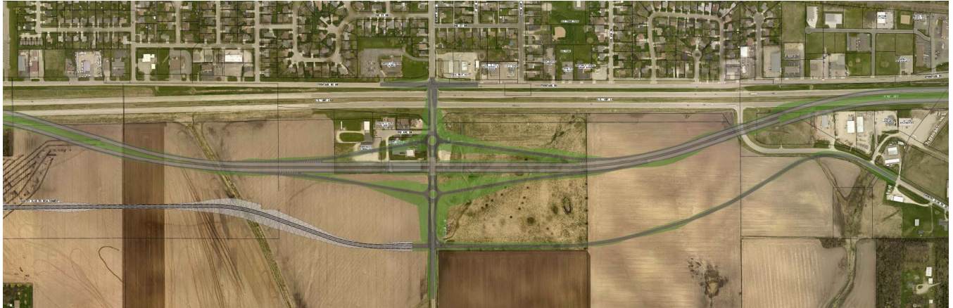
Figure 38. CSAH 5 Conceptual Interchange Alternative – Dual Roundabouts
